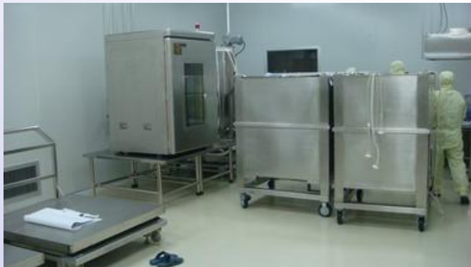
TideCell 100 System during operation. Two 500 L Medium tanks (right) are for perfusion culture.
